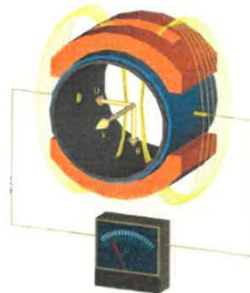
Figure 1: Principle of the electromagnetic flowmeter
